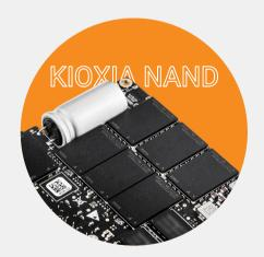
KIOXIA's BiCS FLASH is a three-dimensional(3D) vertical flash memory cell structure. This structure enables it to surpass the capacity of mainstream 2D (planar) flash memory. KIOXIA's TLC 3-bit-per-cell 512Gb(64GB) BiCS FLASH, an industry first, enhances the reliability of write/erase endurance while boosting write speeds.
